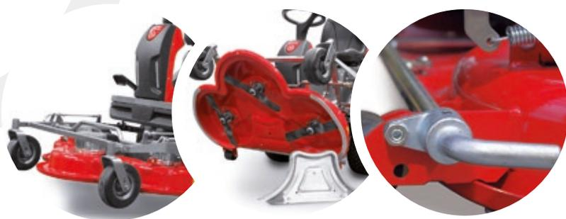
GSR+ Electric also enables **REAR DISCHARGE** option. This function can be obtained by simply removing a mulching plug placed under the mower deck, thanks to the operation of a conveniently placed lever on the right side (driver's side) of the mower's deck.
